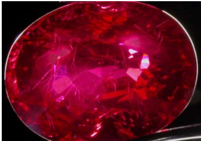
Fig. 3: Ruby from Winza, Tanzania. Characteristic inclusions consist in fine bent fibers with a polycrystalline filling of probably secondary minerals. Photo © H.A. Hänni, SSEF Swiss Gemmological Institute
