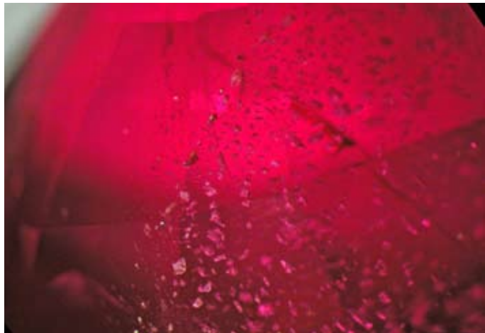
Fig. 4: Ruby from Winza, Tanzania, with a healing fissure charged with multiphase inclusions. Photo © H.A. Hänni, SSEF Swiss Gemmological Institute
